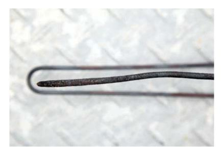
This is a burst core tube from a boiler matrix.
