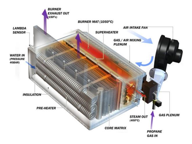
This illustration helps to explain the inner workings of one, of the car 's 12 boilers.
