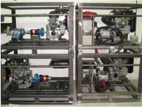
Rig construction continues, this picture shows the two electric rigs and the two water rigs. One of the gas /air rigs is finished and the second is currently in build. We hope to commission the rigs in the next few weeks.
