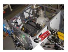
The turbine and final drive is installed. The oil system pipes and pumps are being fitted and the rear suspension is back on the car.
