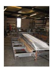
The trolley is complete and looking good with its white PVC cover. It has been tested with 3.5 tonnes of concrete blocks on board. Once we have taken delivery we will fit the trolley with a hydraulic system for raising the car. The trailer is well under way, and should be ready to take the car to its first tests.
