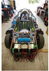
The car is on its wheels and a final fit of the first four boilers with hoses, plumbing and electrics is underway.
