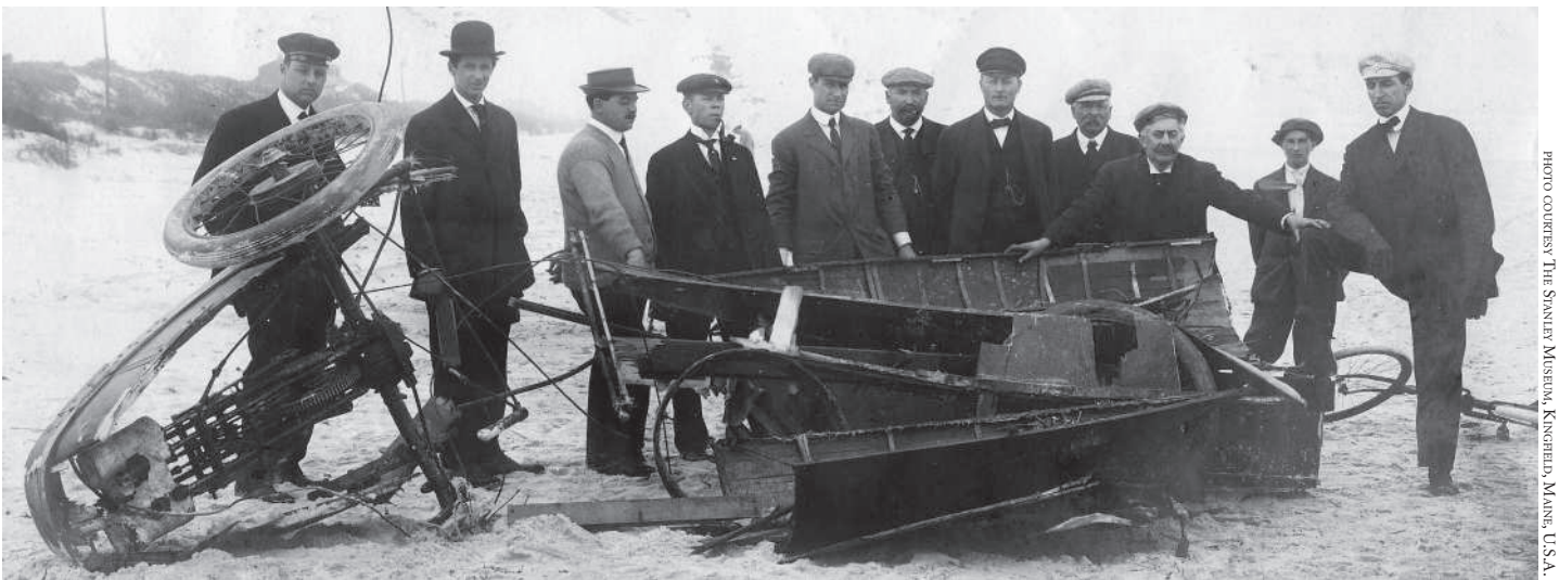
The wreckage of the Rocket was gathered after the crash. Note the ribs visible in the interior of the car body.
